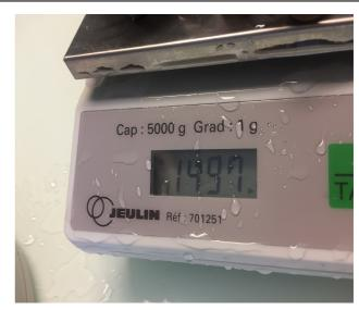
Here is « Shrek ». We made a first prototype with one sheet, it supported 435g. We created a second one, stronger, with 5 sheets ; it looks the same but larger. We assembled the 5 sheets, lined the bottom and folded the four corners. It supported 1497g.
