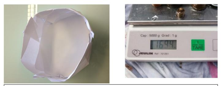
Here is the « Apple Pie ». We made it with 3 sheets : it supported 975g. We tried again with 5 sheets and we had better results : 1694g . For making the second one, we glued the sheets together, folded the edges to make a circle and finally put two sheets for the base of the boat to assure a better rebustness.
